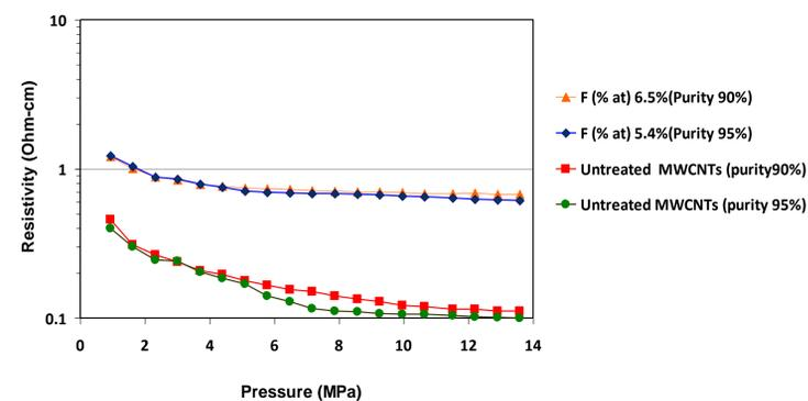
The conductivity measurements evidenced that the conductive properties of the MWCNTs treated with PFPE peroxide were maintained, even if the surface properties significantly changed. These results suggest that the functionalization of MWCNTs with linear PFPE peroxide occurs mainly at the outer tube while the inner tube remains almost unaltered.
