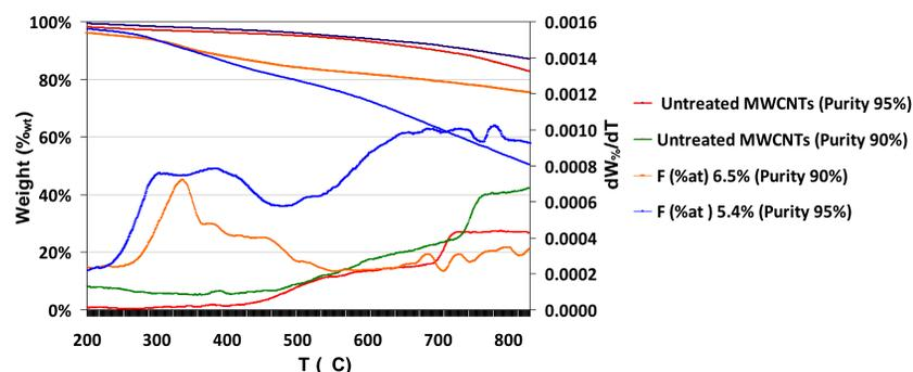
The TGA measurement revealed that the degradation of untreated MW-CNTs started around 450 C. The samples treated with linear PFPE peroxide showed a weight loss in two separated steps: the first weight loss was approximately between 240-450 C and it was due to the degradation of PFPE chains on the sidewall of MWCNTs; a second weight loss started after 450 C and it can be ascribed to the degradation of modified parts of carbon nanotubes.
