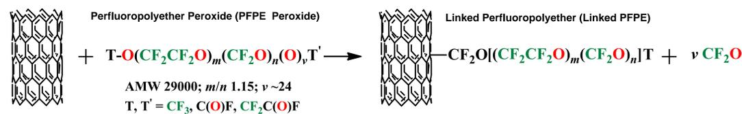
The thermal-induced homolysis of peroxidic bonds in linear PFPE peroxide generates reactive radical species with a PFPE structure, which are able to form covalent bonds on the sidewall of the MWCNTs.
